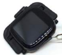
Use SIM Card tool to open up SIM card port
